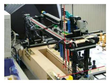
Figure 7.1: Illustrating the different axii the robot must move in
