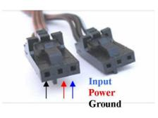
Figure 4.1: Analogue sensor connector for the Phidgets Interface Kit
