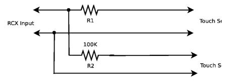
Figure 7.2: Schematic of multiplexer circuit
