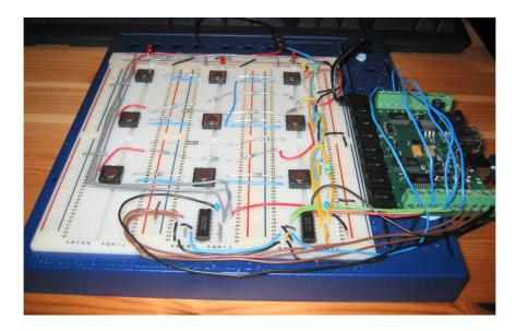
Figure 4.2: The 3x3 Prototype used to prototype the board circuit
