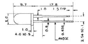
Figure 4.4: Diagram extracted from the LED data sheet
