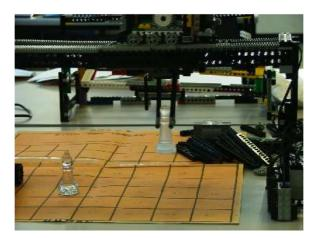
Figure 7.5: The robot moving a glass piece during early testing
