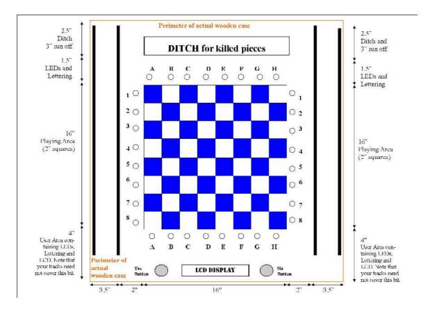
Figure 4.5: Diagram showing the layout of the top of the board
