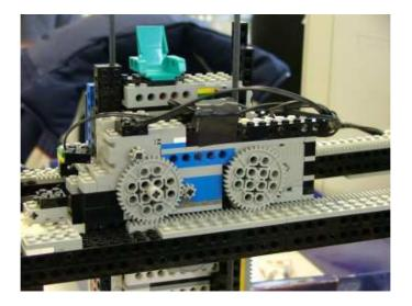
Figure 3.12: Picture of gear train
