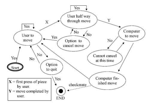
Figure 5.1: State transition diagram for the user buttons
