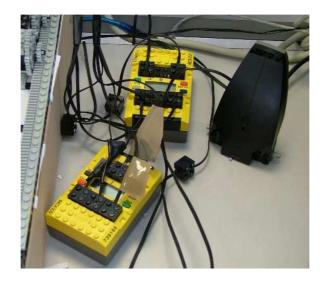
Figure 7.4: The two RCX blocks used, lined up for communication
